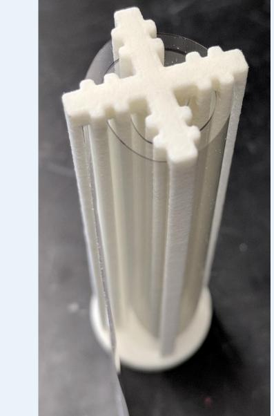
The Rutgers **Electrostatic Passive** Sampler (REPS)
